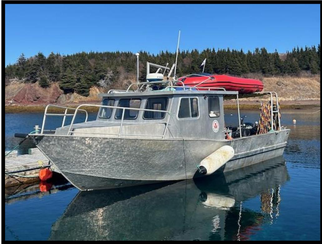
Pro-Dive owns a locally built aluminum hull utility boat that is fitted out for near shore dive operations and to support marine work as required.
